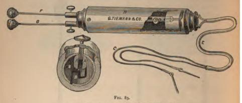
Beard's Current-Reverser, with flexible electrodes.
